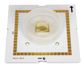
Multi Channel Systems' multi-electrode arrays (MEAs) allow for the recording and analysis of neuronal activity and neural network synchronicity in cell cultures, brain slices, or organoids.
