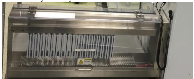
Figure 17. Enclosed and heated output conveyor
